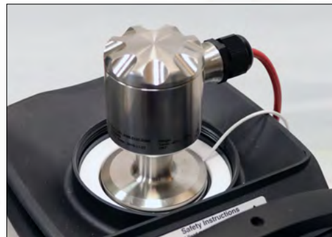
STS-102 A 035 sensor and sanitary sensor in an insert, mounted in an RTC-168 calibrator.
